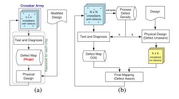
Fig. 6. (a) Traditional defect-aware design flow (b) The proposed defect-unaware design flow
