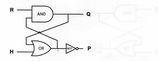
a) An expected operation of the circuit is having complemented logic values for Q and P outputs. Determine the restrictions on R and H so that P equals to Q. Fill in the truth table below with indicating the bad conditions or restricted cases
