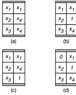
Fig. 2. Four different minimum size switching lattices implementing the function  $f = x_1x_2x_3 + x_1x_4$ . (a) A 0-irredundant, but not 1-irredundant, lattice; (b) a 1-irredundant, but not 0-irredundant, lattice; (c) a fully testable lattice; (d) a fully testable lattice with a minimum number of literals.
