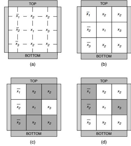
Fig. 1. A four terminal switching network implementing the function  $f = \bar{x}_1\bar{x}_2\bar{x}_3 + x_1x_2 + x_2x_3$  (a); its corresponding lattice form (b); the lattice evaluated on the assignments 1,1,0 (c) and 0, 0, 1 (d), with grey and white squares representing ON and OFF switches, respectively.
