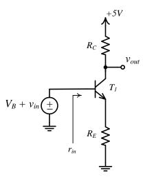
Common Emitter Amplifier with an Emitter Resistance
