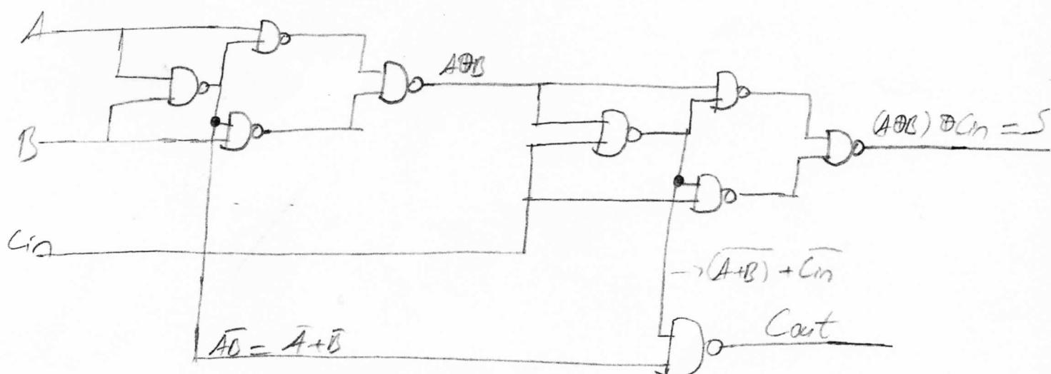
f) i) Construct using two half adder;
