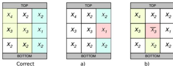
The cell  $c$  in a) is essential and the CF is testable, the cell  $c$  in b) is not essential and the CF not testable.
