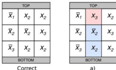
The blue subpath is unsatisfiable, so  $\text{CF}(c, x_2, x_3)$  cannot be tested.
