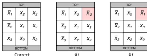
a)  $\text{CF}(c, x_2, \bar{x}_2)$ , b)  $\text{CF}(c, x_2, \bar{x}_1)$ . a) is testable with test vector  $\bar{x}_1 x_2 x_3$
